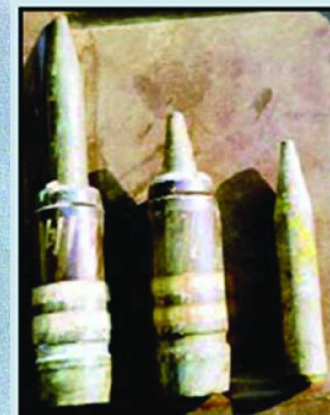
30mm DU munition: jacket and penetrator
